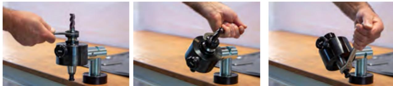
Turn your tool at any time within seconds into the desired position. Ergonomic and healthy working conditions thanks to the **practical rotating function**.
