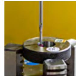
Position the tester approximately on the centre of the circle. Preselect if you want to probe inside or outside and give an approximate diameter. After starting, the cycle automatically probes in X axis, Y axis and automatically writes into the offset - that's it!
