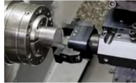
Position the bar gripper in Z axis in front of the bar.
