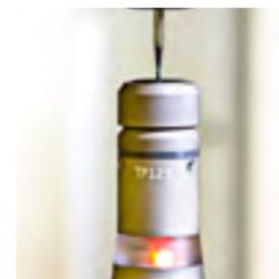
Chose the milling tool you want to check and start the cycle. After starting, the cycle automatically probes the tool length. If the tool is broken, the cycle does not find any probing signal and stops the machine. Additionally, you can preselect a confidence range as a tolerance. Is the tool out of tolerance, the machine stops. Otherwise, the machine goes on working.
