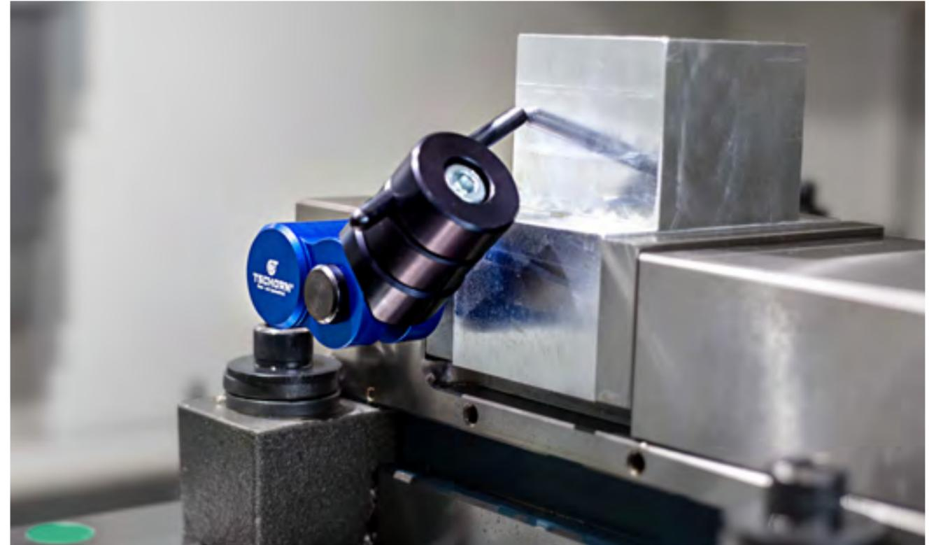
With its built-in magnets the workpiece stopper gets fixed directly to a bench vice (for example) and applies for exact positioning of your workpiece. After clamping, it can simply be removed and releases the positioning surface for processing.
