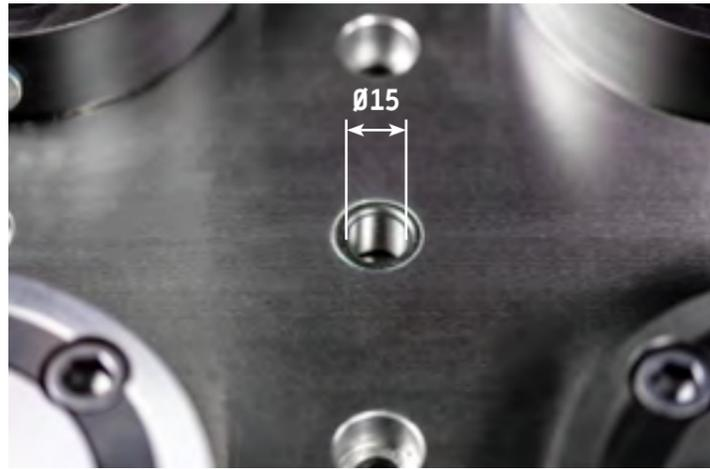
Thanks to the probing bore hole, the centre position of the zero clamping system can be determined extremely quickly and easily.
