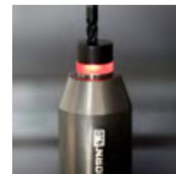
Chose the milling tool you want to measure and start the cycle. After starting, the cycle automatically probes the tool length and writes the tool length into the tool offset of the machine.
