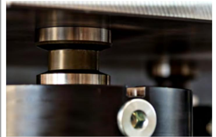
The locating bolts have two different diameters. The lower one is used for easy insertion and the upper one for exact positioning.
