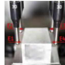
Position the tester in the X axis in front of the edge. Preselect the edge 1, 2, 3 or 4. Start: the cycle automatically measures first X, then Y, then Z, and automatically writes all axes into the offset - that's it!
