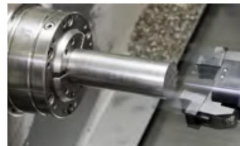
Move the bar gripper in Z direction off the bar and start machining.
