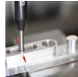
Position the tester approximately on the centre of the slot or the key. Then you chose if you want to measure inside or outside, preselect the axis and give an approximate width. After starting, the cycle automatically probes the centre in the X axis or Y axis and automatically writes into the offset - that's it!
