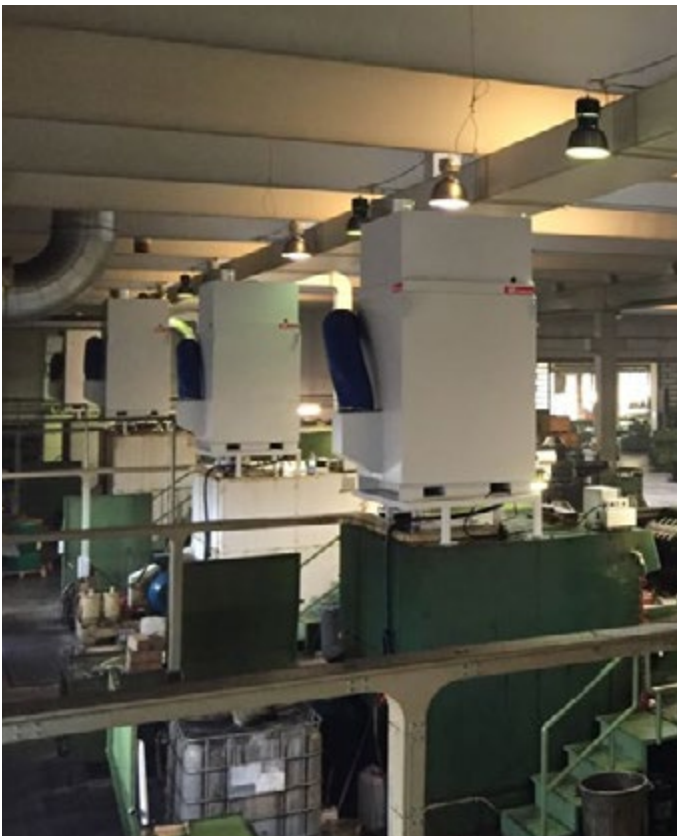
AR 10.000 installation on SACMA automatic presses
