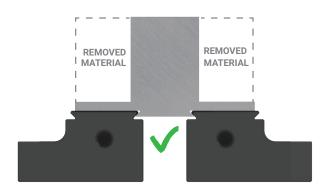
For narrow parts, position the dovetail as close as possible to the **finished part's** center of mass.
